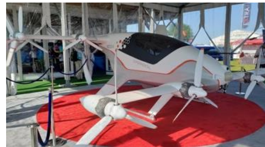
Figure 37. The A3 Vahana single-seat autonomous demonstrator eVTOL aircraft is the forerunner for an Airbus air taxi short-range aircraft for urban air mobility (UAM). Image courtesy of Johnny Doo
